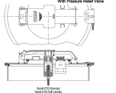
PAF Manholes with Model PAF450 10" Pressure Relief Valve are certified for use on MC306 cargo tanks. Manholes are certified and marked in accordance with 49CFR178.345-5 with test pressure of 36 psig.
